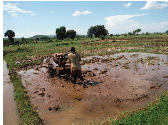
Photo41 Some farmer have small paddy field like this. In this circumstance, power tiller can be more competitive than big tractor.
