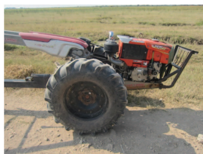
Photo III.3.1 Installed large tires
