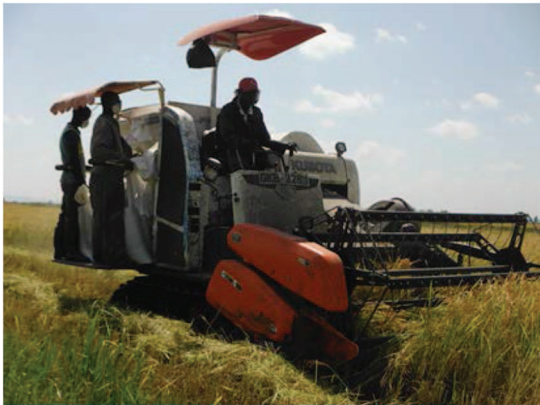
Photo14 Harvesting and Threshing by machinery. The project choose a combine harvester for comparison. This is KUBOTA DC-70
