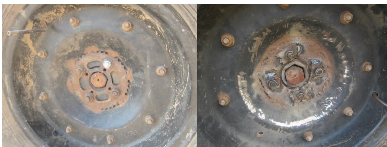
Photo III.3.2 and III.3.3 Rim reinforcement
