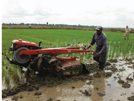
Photo4 Ploughing by power tiller. Cautious approach is necessary to manage on black cotton soil.
