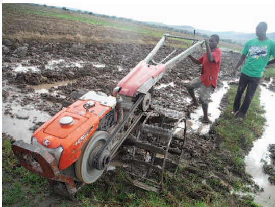
Photo39 The power tiller after ploughing activity. Its modified bumper was so characteristic.
