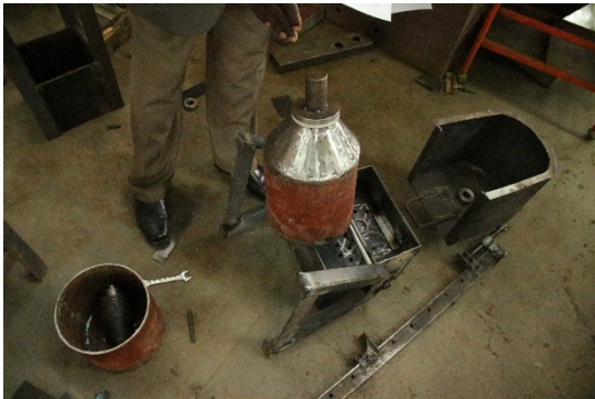
Photo 7 Trial production of a pressure popping machine in the city (JKUAT).
