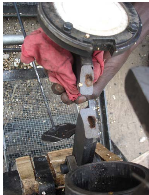
Photo 1. Part broken due to the inadequate strength. It shows a large air bubble in the part that was produced by the foundry technique. Manufactured by DK Engineering.
