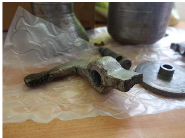
Photo 4. Broken piece of the lid section (cast iron).
