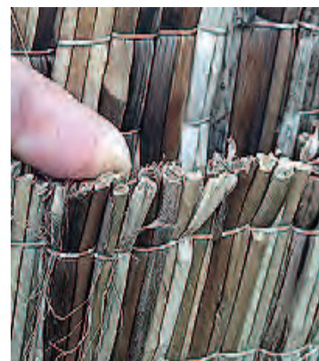
Single-layer mat made of the stems of cattail and giant bulrush
