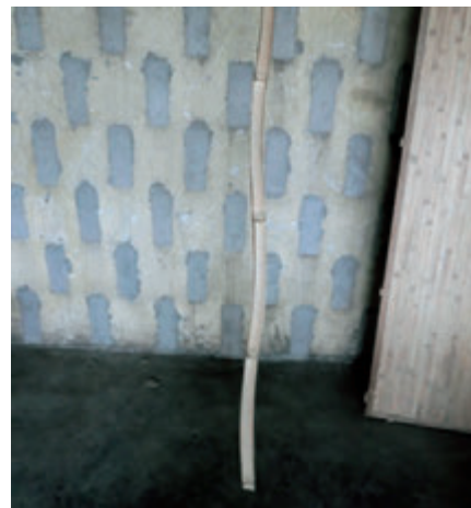
Photograph 3-1-37: Roughly cracked bamboo. Substantially bent.
