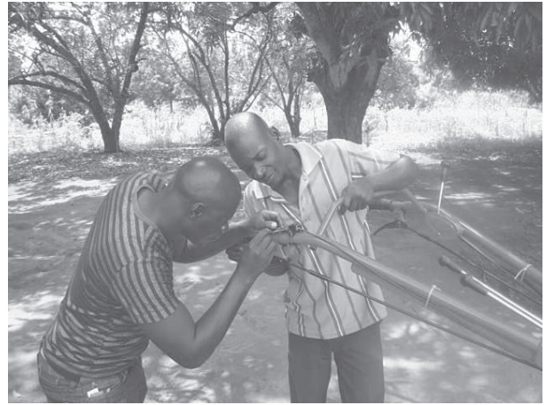
Photo 4: A staff from 3WM trying to repair accelerator cable after delivering PT.
