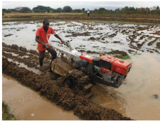
Photo5 Puddling with power tiller (Rotavator plot)
