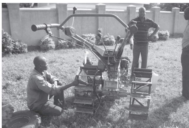
Figure 9: Trainees fixing cage wheels
