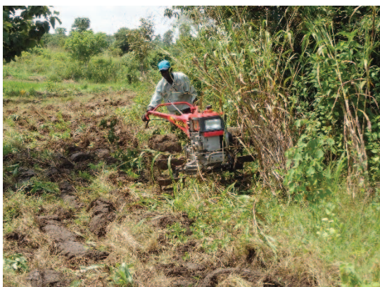
Photo14 Trial by a rice farmer in Lira District. Power tiller made ploughing easier even in the field overgrowned by weed.
