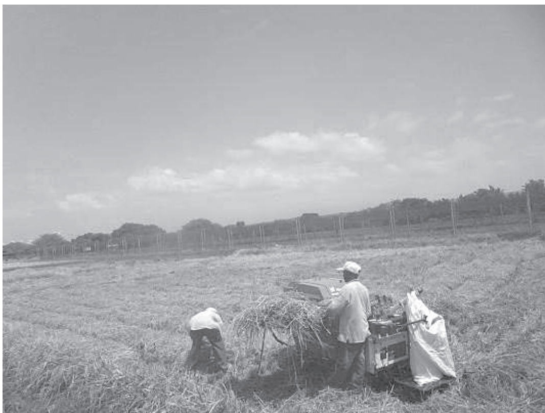
Figure 22 Threshing rice by rice thresher (two people required collecting crop and feeding the machine)
