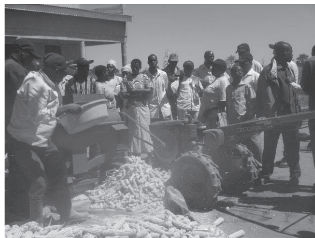
Figure 3b: Farmers shell Maize with Power tiller
