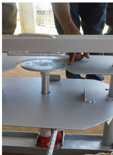
Photo 100, 101 Demonstration of a puff cracker machine in Itumbu rural group in Vihiga Country at the West of Kenya (left). Puff-cracker machine delivered by DK Company. (right). The space between the disc at the center and the iron bench is not even, requiring adjustments.
