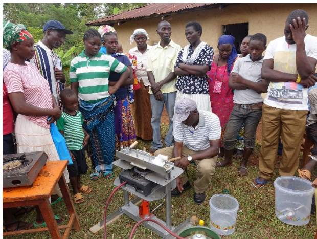
Photo 100, 101 Demonstration of a puff cracker machine in Itumbu rural group in Vihiga Country at the West of Kenya (left). Puff-cracker machine delivered by DK Company. (right). The space between the disc at the center and the iron bench is not even, requiring adjustments.
