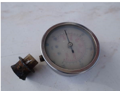
Photo 15, 16 Pressure gauge with coupler joint, broken by strong shock at striking (Left) and pressure gauge removable at striking not to receive shock (Right)
