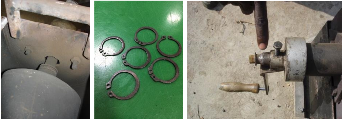
Photo 6, 7, 8 The handle attachment pin comes off and the cylinder is slid forward (left and center). Since the shaft pin could not be repaired, the part was welded directly (Left). DK Engineering deepened the pin grooved so that the pin would not come off.
