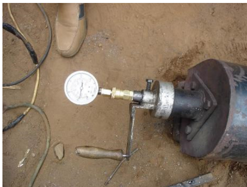
Photo 15, 16 Pressure gauge with coupler joint, broken by strong shock at striking (Left) and pressure gauge removable at striking not to receive shock (Right)
