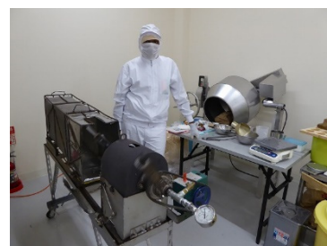
Photo 76 Pressure popping machine installed on the work bench
