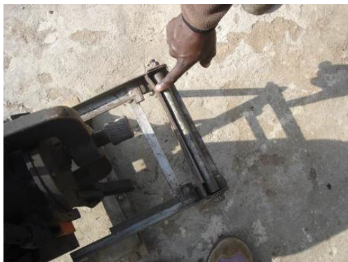
Photo 13, 14 Broken cage (Left) and frame bent by strong shock at striking (Right)
