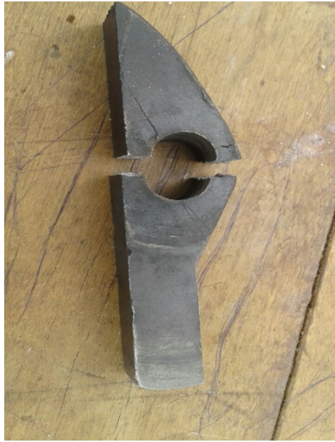
Photo 11, 12 Thread-crushed U shaped part (Left) and broken peg of low strength (Right)
