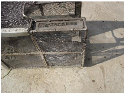
Photo 13, 14 Broken cage (Left) and frame bent by strong shock at striking (Right)
