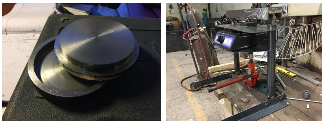
Photo 93, 94 Iron plates for producing puff crackers, manufactured by Numerical Engineering (left), and prototyping of puff-cracker machine (right) from DK Engineering. A gas cooker with a hole at the center and a second-hand hydraulic jack for automobiles are used.
