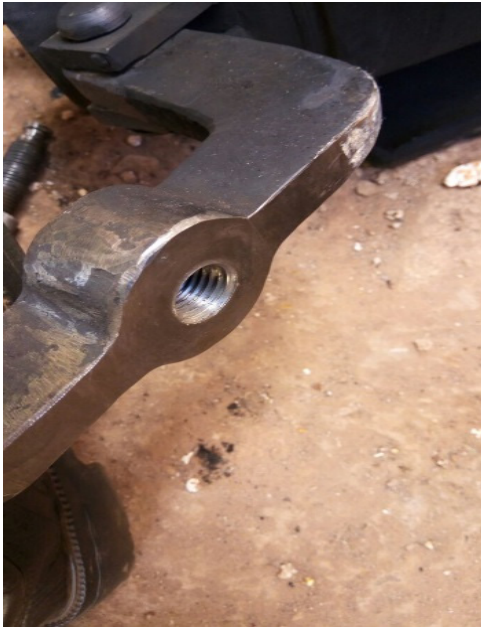
Photo 11, 12 Thread-crushed U shaped part (Left) and broken peg of low strength (Right)
