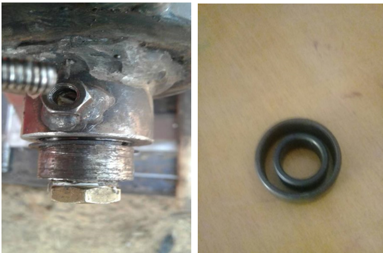
Photo 9, 10 Thread-crushed handle attachment part (Left) and Z bearing of handle completely broken by heat and shock (Right).
